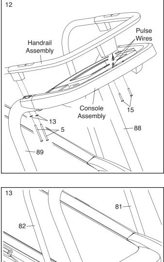
13. Attach the Left and Right Handrails (81, 82) to the Base (91) with four 3/8" x 2 1/8" Patch Bolts (14) and four 3/8" Star Washers (13) (only one side is shown); **do not tighten the Patch Bolts yet.**
